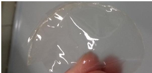
Figure 3.9: Photo of CS1 film fabricated by solvent-casting method
