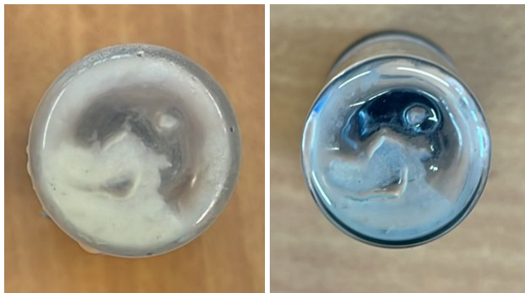
Figure 5.16: Photos of SiGu-sPEG_2 before (left) and after (right) thermal treatment at 70°C
