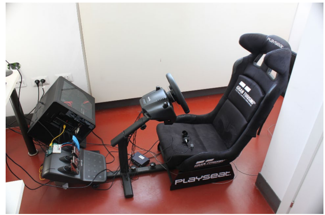
Fig. 2 Experimental setup consisting of a driving seat, a steering wheel and pedals
