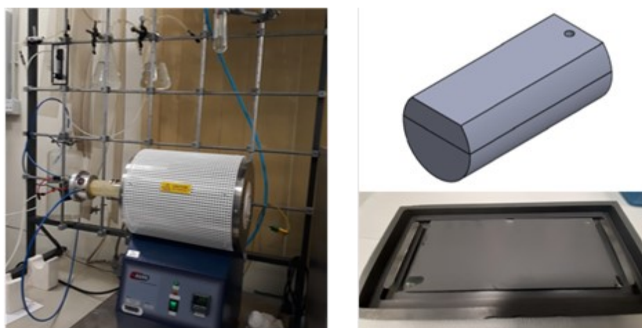
Figure 39: a) Photo of the sulphurisation setup; b) digital design of the graphite box and c) accommodation of a large kesterite sample (3.5x7 cm 2 ) inside the box.
