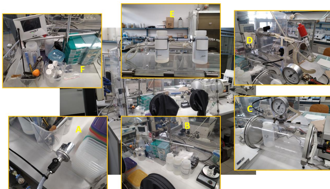
Appendix 3 - Details of wet box: a) double check valves on the in-gas line of wet box, b) workbench, c) pre-chamber, d) needle valve on the out-gas line of the wet box, e) gases trap, f) AMI 100 carbon dioxide detector
