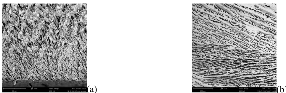
Fig. 1. Micro-images of the (a) cross-section and (b) top YSZ backbone after sintering at 1400 °C.
