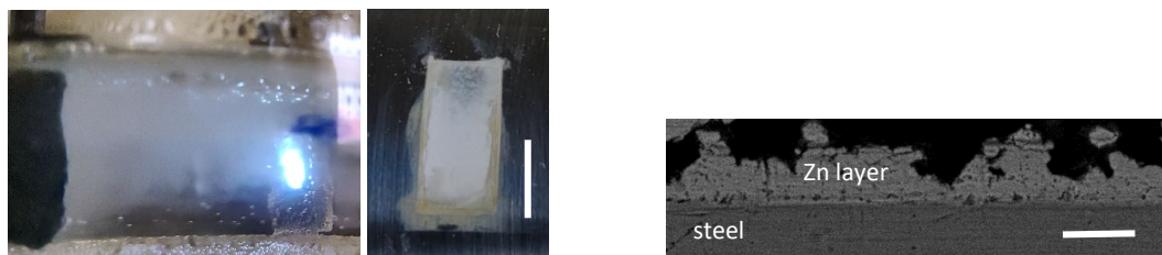
Figure 1. Left: electrolytic plasma regime in 1.3 M \text{NH}_4\text{Cl} solution and effect of the treatment on a steel plate (marker = 0.5 cm). Right: BS-SEM micrograph of a cross section after CPE galvanizing (marker = 10 \mu\text{m} ).
