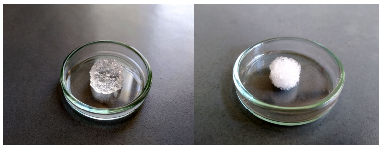
Figure 1. Images of a scaffold functionalized with GLI: wet (left) and lyophilized (right).
