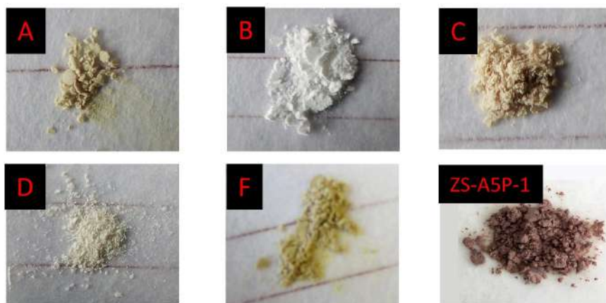
Figure 5.3: Digital pictures of some samples from different batches of one porphyrin functionalized ZnO/SiO 2 nanosystem (ZS-A5P-1) after centrifugation in PBS dispersions, compared to the sample as synthesized.
