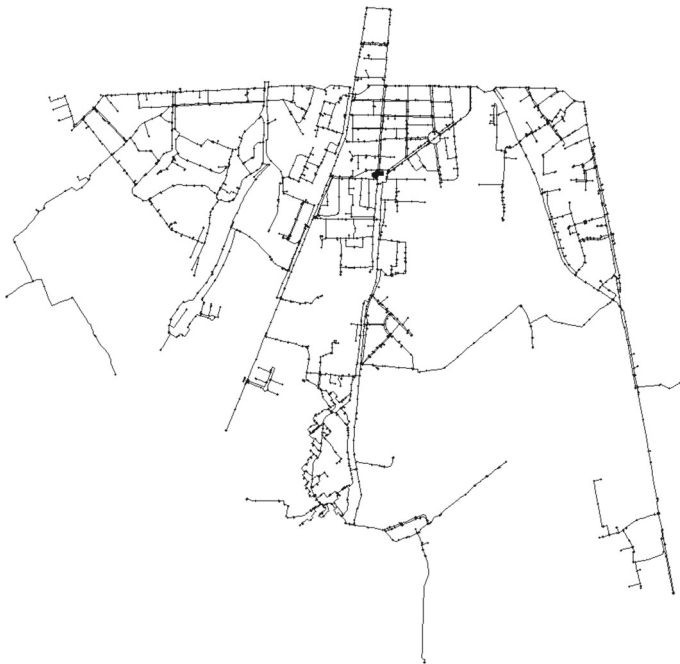
Fig. 5 EPANET model of the Pressure Management Zone (PMZ) “Abbiategrasso”, in Milan, Italy
