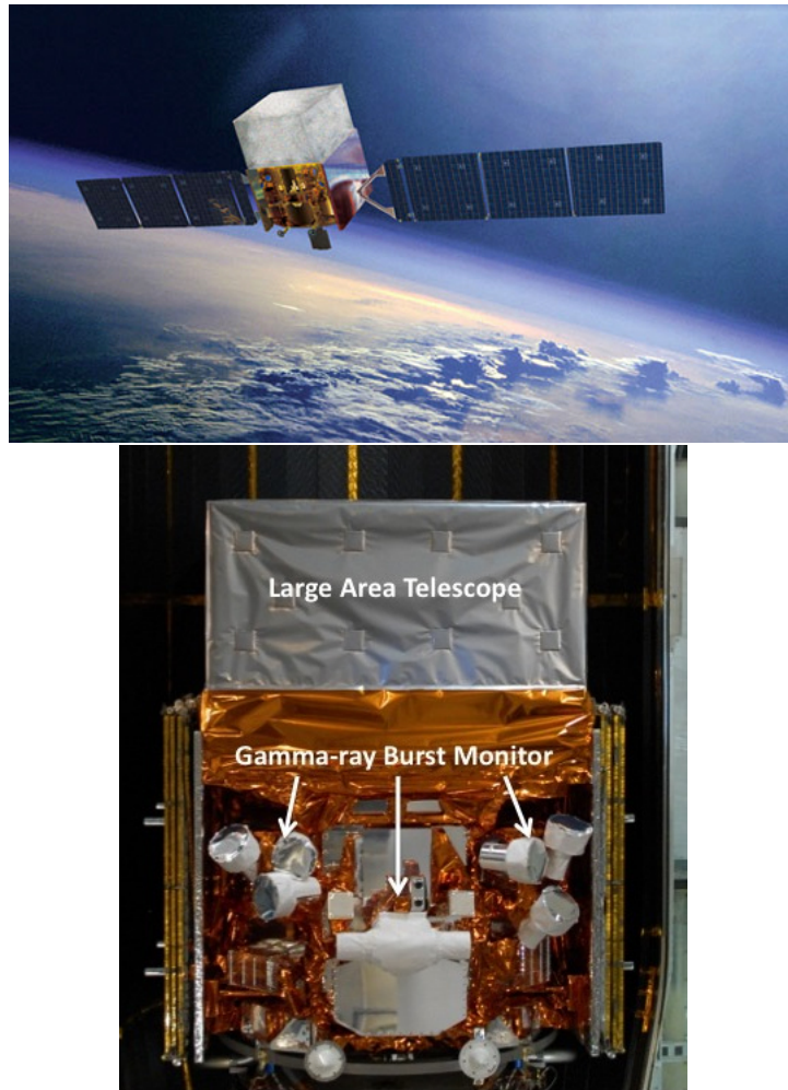
FIGURE 2.12: Top: artistic representation of the Fermi satellite in space. Bottom: the two instruments of the Fermi satellite (labeled in white) assembled together and prepared for the launch. Credit: NASA ( https://fermi.gsfc.nasa.gov/science/eteu/about/ )
