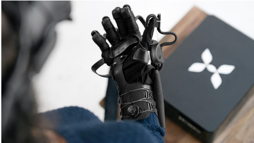
Figure 1. Realistic sensory-motor interactive virtual worlds in virtual reality: Haptic gloves let the user feel virtual objects and perform actions with high fidelity to reality (HaptX, 2017).
