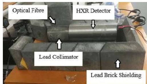
FIGURE 4.5: REGARDS at COMPASS. The HXR detector is placed inside the soft iron magnetic shielding cylinder. A 10 cm lead collimator is placed in front of the detector. Lead bricks are used to shield the detector from background radiation.
