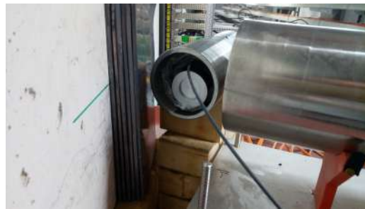
FIGURE 4.7: REGARDS HXR detector at AUG. Six lead sheets are placed in between the spectrometer and the line of sight to attenuate the HXR flux.
