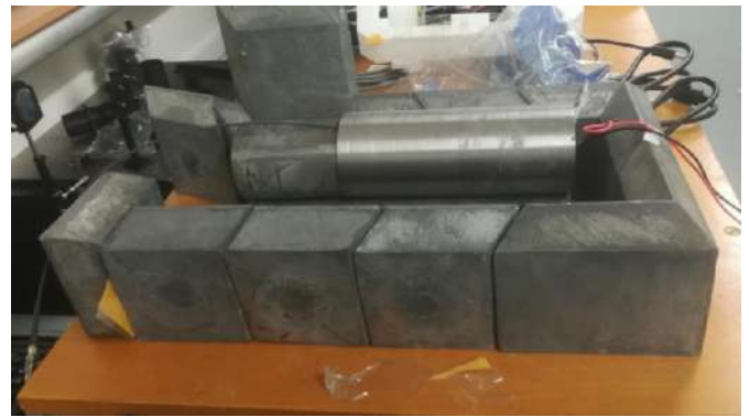
Figure 13. REGARDS detector setup at COMPASS. At the centre of the picture the soft iron pipe for magnetic shielding is visible. At its left, the cylindrical lead collimator and the black optical fibre are visible. Lead bricks were used to shield the detector from the background radiation.
