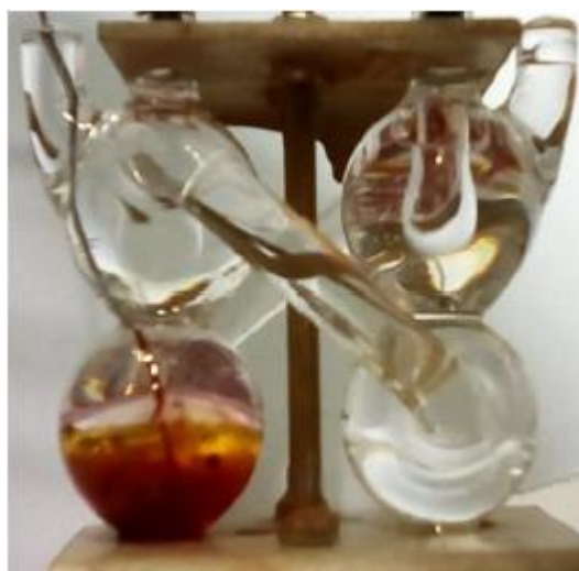
Figure 5.27. TLE during the injection of iodine solution in the left side. The bottom of TLE is filled with two water solution of NaI (1M on the left and 2M on the right). The device is then filled with toluene.
