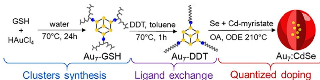
Figure 3.1. Schematics of the three-step synthesis strategy of quantized-doped Au:CdSe NCs. First, water-soluble \text{Au}_7 -clusters were synthesized by chemical reduction of the metal precursor \text{HAuCl}_4 using glutathione (GSH), which also acts as capping ligand. Second, the clusters were phase-transferred from water to toluene by exchanging strongly polar GSH molecules with nonpolar 1-dodecanethiol (DDT) molecules. Finally, Au:CdSe NCs were seeded-grown using the \text{Au}_7 clusters.
