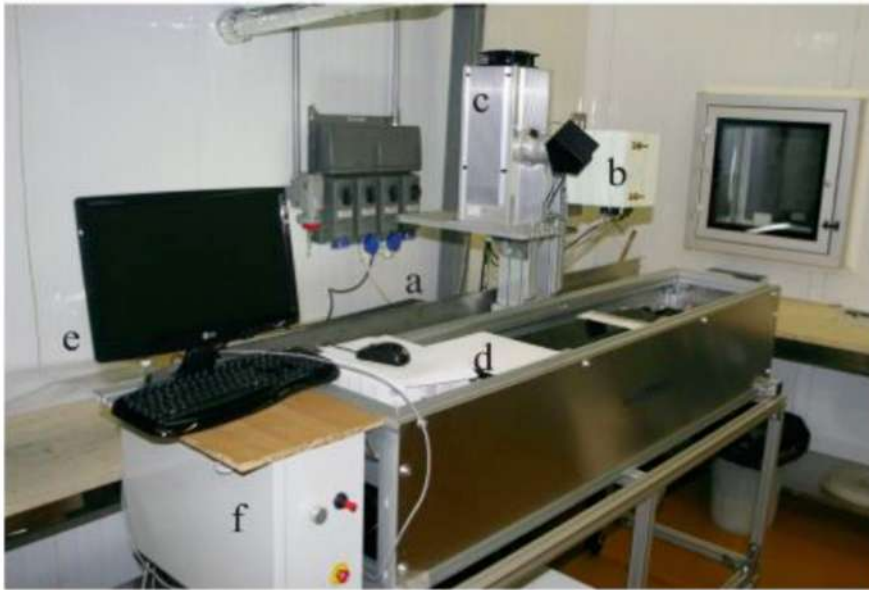
Figure 11. Picture of the system used to acquire the hyperspectral imagery. The system consists of: (a) samples holder and motor driver; (b) HeadWall VNIR camera thermostated by heaters; (c) stable halogen lamp; (d) calibrated Lambertian Spectralon panel; (e) PC connected to the spectrometer by a dedicated interface.
