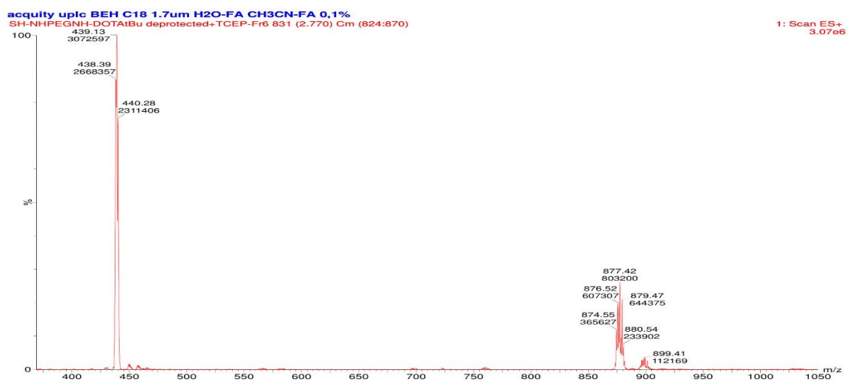
Figure 12 ESI-Mass spectrum of Gd(III) complex 6. Calculated m/z for C_{30}H_{52}GdN_7O_{11}S = 877.3 , found m/z for C_{30}H_{52}GdN_7O_{11}S = 877.4 (M+H)^+ , 439.1 (M+2H)^{2+}
