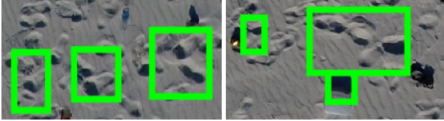
Figure 5.8. Examples of shadows in the proximity of footprints (left image) or of AMD (right image), that are mistaken as AMD by the software, representing pitfalls for the algorithm in its present version.
