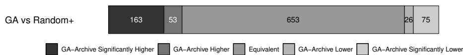
Fig. 14: Comparing the coverage achieved by GA against Random+ over the 970 SourceForge classes, with archive enabled: Compared to Figure 3, the archive of solutions is an effective way to increase the performance of GA , however, for a large number of subjects, the evolutionary and random techniques perform similarly.
