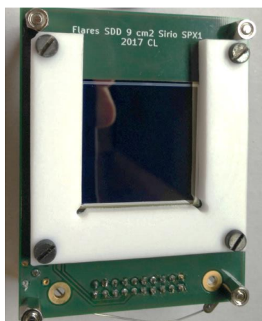
Figure 5.17: Picture of large area SDD mounted on the holder.
