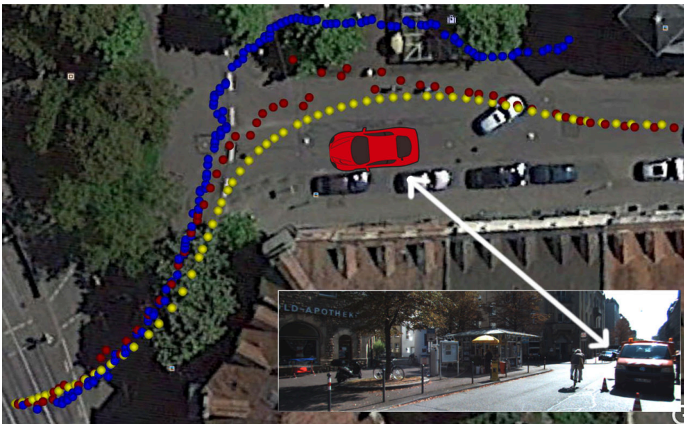
Figure 5.6: The trajectory for the 2011_09_26_drive_0005 sequence. Yellow points are the ground truth positions, red points are the position estimates of our proposal, blue points are the position estimates of the baseline algorithm. The red car is associated to the parked truck visible in the overlaid camera frame.
