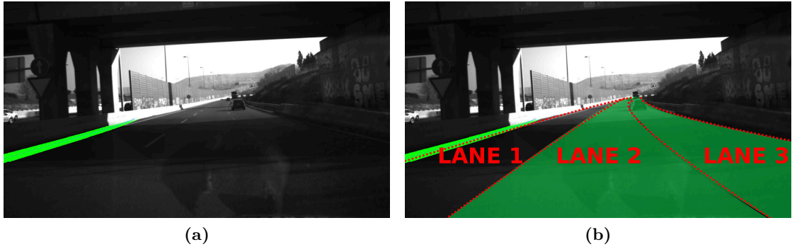
Figure 3.2: In (a) only one line out of four is detected, thus the highlighted lanes in (b) have a higher probability of being the vehicle ego-lane, as implicated by the distances to the detected lines.
