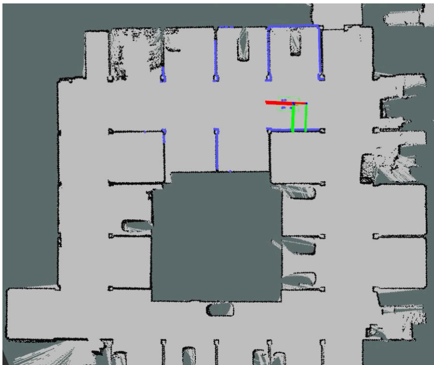
Figure 2.2: A bi-dimensional grid map of the environment where gray pixels represent free space, black pixels represent obstacles and teal pixels represent unknown areas. The LiDAR scan at the estimated robot position is shown in blue. The good alignment of the measures with respect to the map indicates a good localization estimate.
