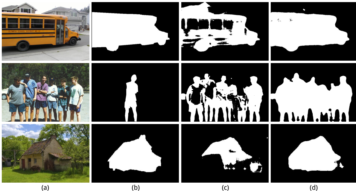
Fig. 3.6 Effect of multiscale analysis on example images: input image (a), ground truth annotation (b), single-scale saliency estimation (c), and multiscale saliency estimation (d). The content of columns (c) and (d) is here binarized to facilitate the comparison.
