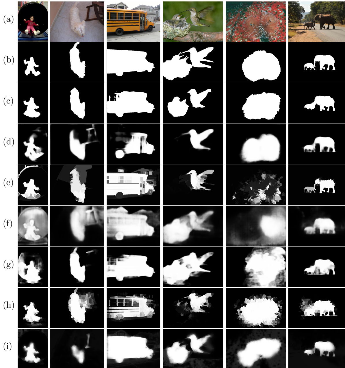
Fig. 3.9 Visual results of the extended CNN from DL-MAE . Rows (a) and (b) show, respectively, the starting image and the corresponding ground truth annotation. (c) is the output of DL-MAE . Rows (d) to (i) are the input saliency maps used by DL-MAE , namely: (d) DSS, (e) MDF, (f) MFCN, (g) DHS, (h) ELD, (i) RFCN.
