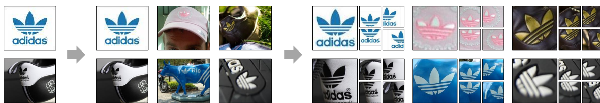
Fig. 6.8 Visualization of the joint contribution of both real data augmentation (obtained through the collection of the Logos-32plus dataset) and synthetic data augmentation (obtained with random translation).
