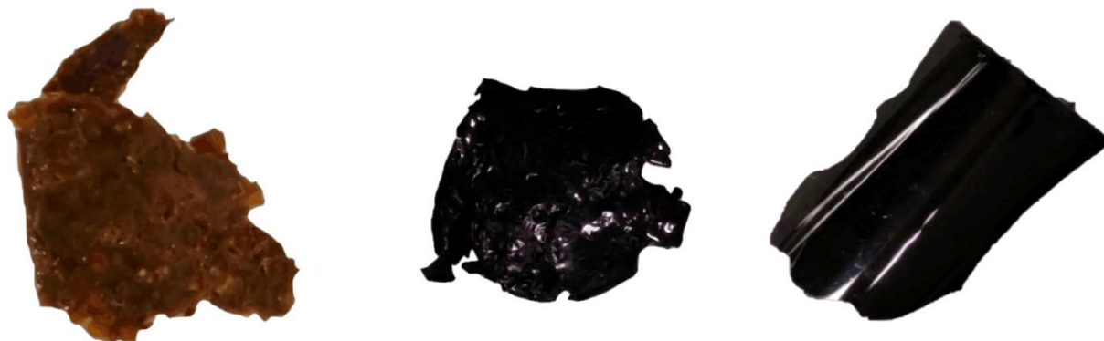
Figure 4.11 On the left: pNTEC 12 T 2 before thermal treatment; in the center: pNTEC 12 T 2 after thermal treatment with p-toluene sulfonic acid at 180°C, under N 2 for 2h; on the right: pNTEC 12 T 2 after thermal treatment at 400°C, under N 2 for 20 minutes
