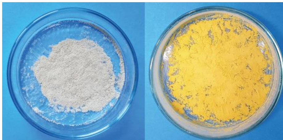
Figure 4.7. PSF2 before (left) and after (right) exposure to 365 nm light for 24 hours.
