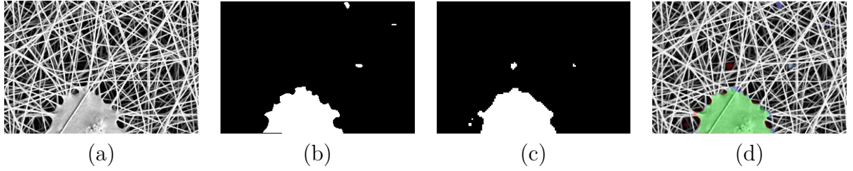
Fig. A.4 (a) The input image \mathbf{I} . (b) The binary mask of anomalies \Omega_{\mathbf{I}} . White pixels represent anomalies. (c) Estimated mask of anomalies \widetilde{\Omega}_{\mathbf{I}} . White pixels represent anomalies. (d) Difference between \Omega_{\mathbf{I}} and \widetilde{\Omega}_{\mathbf{I}} overlaid on the test image. Green pixels represent true positives , red pixels represent false positives , blue pixels represent false negatives , no color pixels represent true negatives .
