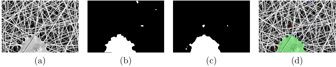
Fig. 6.3 (a) The input image \mathbf{I} . (b) The binary mask of anomalies \Omega_{\mathbf{I}} . White pixels represent anomalies. (c) Estimated mask of anomalies \widetilde{\Omega}_{\mathbf{I}} . White pixels represent anomalies. (d) Difference between \Omega_{\mathbf{I}} and \widetilde{\Omega}_{\mathbf{I}} overlaid on the test image. Green pixels represent true positives , red pixels represent false positives , blue pixels represent false negatives , no color pixels represent true negatives .
