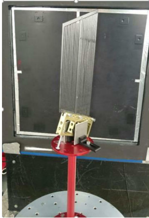
Figure 5: Setup of the neutron radiography with the aluminum grid installed on the rotation stage.
