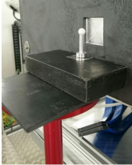
Figure 2. Setup of the experiment on IMAT. The sample is placed in front of the MCP detector and exposed to the neutron beam for eight hours.
