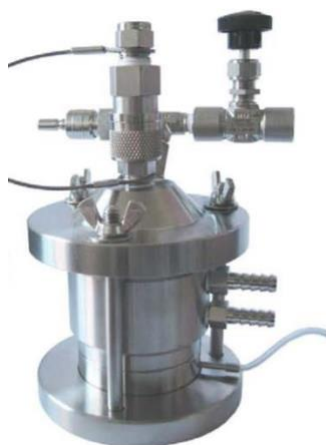
Figure 2: Liposome membrane extruder (Avanti Polar Lipids)
