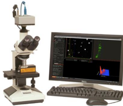
Figure 9: Nanosight instrument for the detection of size (nm) and aggregation
