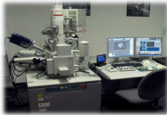
Figure 15: Scanning Electron Microscopy SEM system displaying the microscope and software for the detection of morphology and topology of nanoparticle surface
