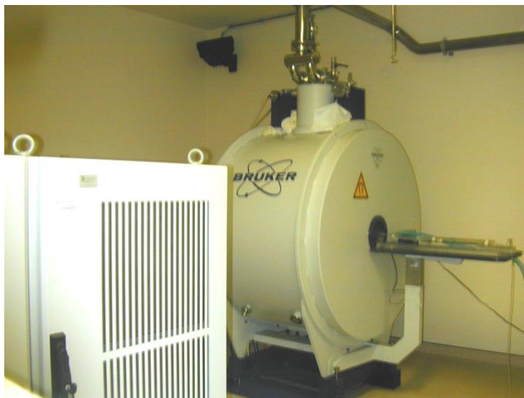
Figure 10: Bruker Pharmascan 7.0 T MRI instrument at Nerviano Medical Sciences (NMS)
