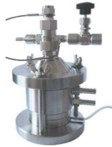
Figure 31: extruder used for the formation of uniform liposomes
