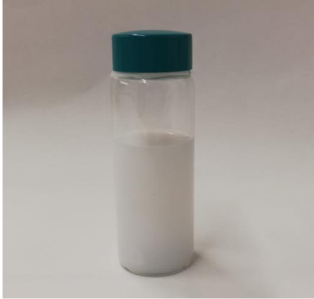
Figure 2-11. Polyisoprene latex with silica particles via Pickering emulsion.
