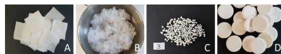
Fig. 1: Production of tablets made from paper. A: paper prior to processing, B: production of pellets, C: pellets made from paper, D: tablets made from paper pellets and with continuous production mode.
