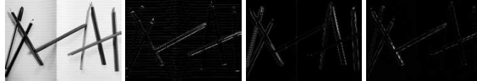
Figure 5: Two level decomposition of the image in Figure 6a using Daubechies wavelet of order 2. The 4 images are the scaling coefficients c^2 and details coefficients along the horizontal, vertical, diagonal direction, from left to right.
