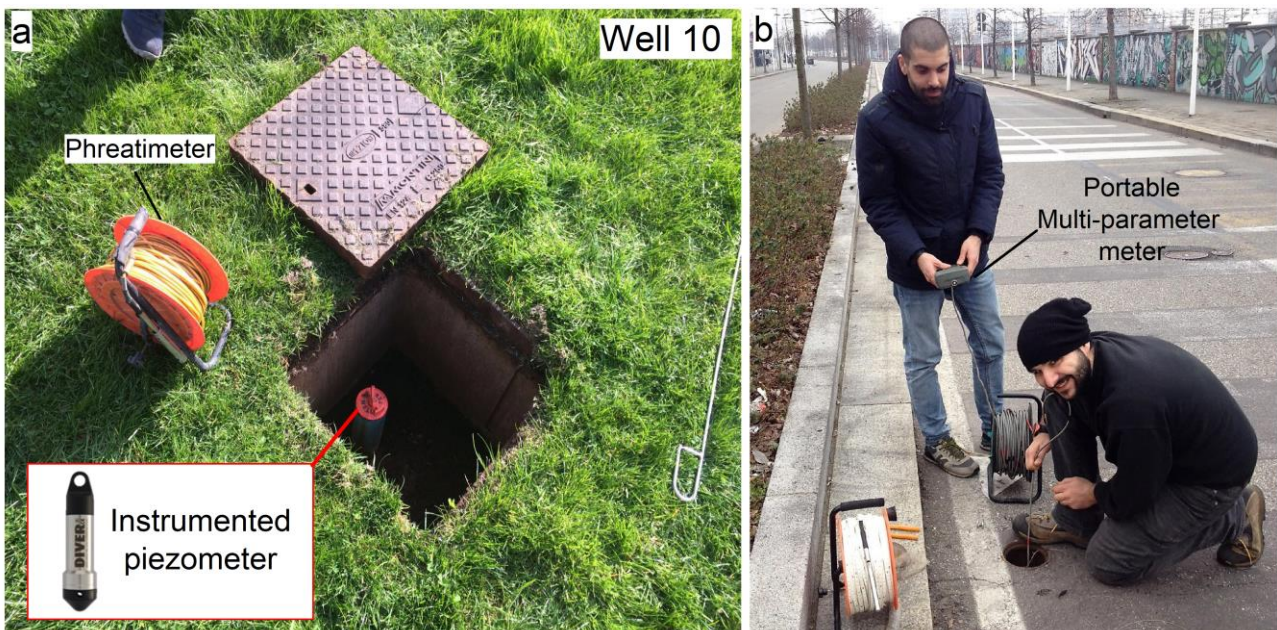
Fig. 2.6 – (a) Example of open-pipe instrumented piezometer (well 10, see green dots in Fig. 2.4 for location) with submersible transducer. (b) Example of temperature-depth manual measurement by means of portable multi-parameter meter.
