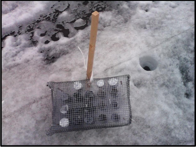
Figure SI-4.2 One rack containing bottles used for microcosm experiments on the surface of Forni Glacier. Racks were covered with a plastic net and bound to a wooden stake drilled into the ice to avoid bottle overturning and dispersal.
