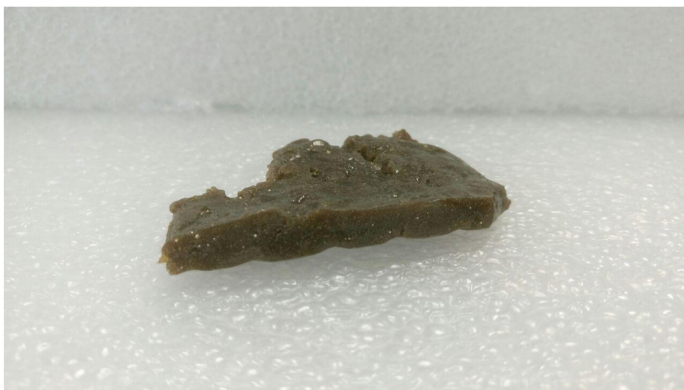
Figure 48 - Unvulcanized blend sample. The visible white dots result from capsule segregation.
