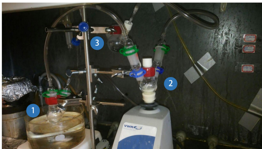
Figure 46 - Working scheme for vapor-phase silanization of TECO2: (1) silane supply; (2) reaction chamber; (3) purging flask
