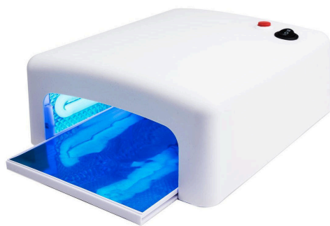
Figure 4.17 “Nail-lamp” (UV-A) setup used for micellar polymerizations.
