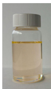
Figure 5.19 Picture of an as-prepared dispersion of \text{PbI}_4(\text{PDMS-NH}_3)_2 nanoplatelets (on the left), and its absorption and PL spectra (on the right)
