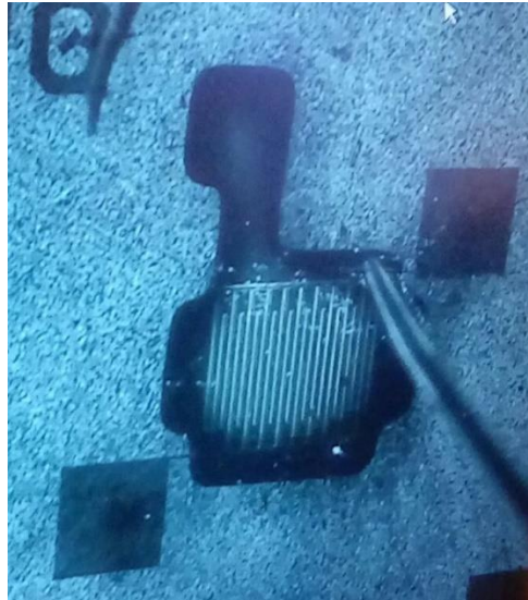
Fig. 4.3. Microscope image of a complete device with a very thin layer of semiconductor. A measuring probe is seen touching the gate contact.
