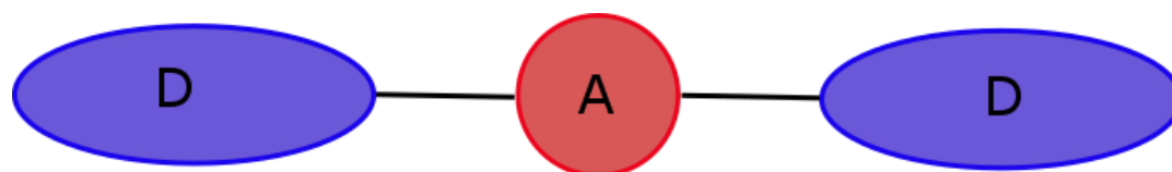
Fig. 1.9. General structure of donor-acceptor small molecule. Donor moiety (blue) is connected by a conjugated bridge to core with acceptor like character (red).
