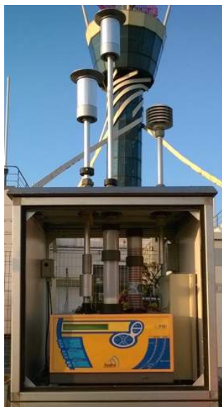
Figure 2.4 Low volume Hydra Dual Channel Air Sampler (gravimetric sampler, FAI)
