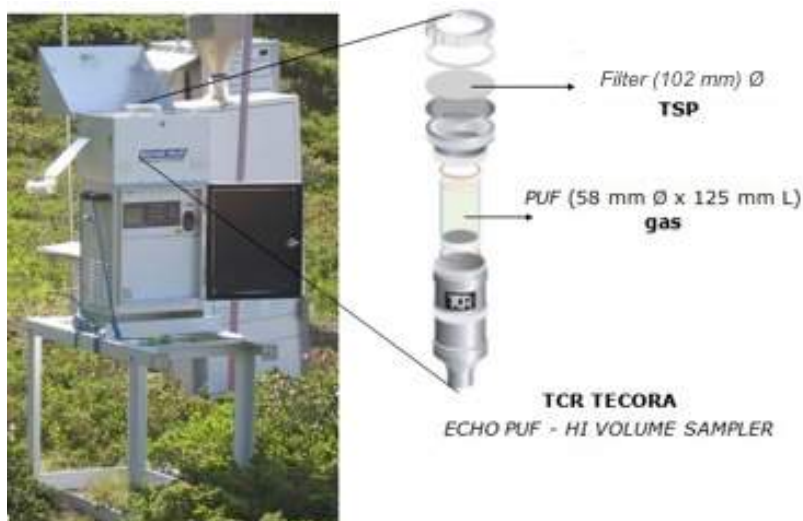
Figure 2.2 High Volume Echo PUF (TCR Tecora); scheme of the filter and PUF lodging.
