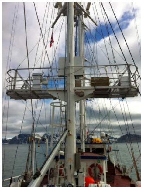
Figure 2.6 Echopuf sampler on board of the oceanographic ship OCEANIA
