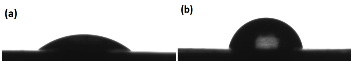
Figure 5.4: Shape of the water drop on film of (a) pristine CNC and (b) functionalized CNC
