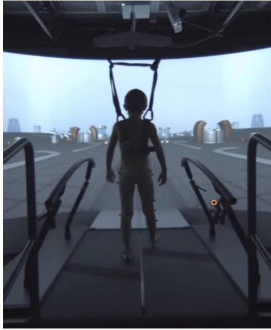
Fig 1.2. Picture of the experimental setup. The participants were instructed to walk barefoot at their own natural speed following the street in front of them presented on a speed-matched virtual environment with 180° projection. Children wore a safety harness over legs and shoulders loosely hanging from the ceiling, to prevent injury in case of an accidental fall. The safety harness did not support body weight during walking.
