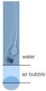
Figure 3.11: Zebrafish embryo immobilized in FEP tubing - schematics.
