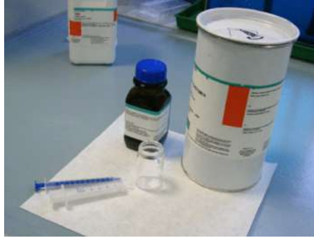
Figure 3.2: Sylgard 184 silicone elastomer consisting of 0.1 L curing agent and 1 L base
