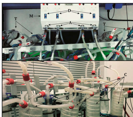
Figure 1. The Vaping machine, custom-made apparatus for generating and condensing vapors from e-CIGs. In the picture it is showed the four channel vaping machine (M) set with four atomizers (A) through 510 socket adapter. Each atomizer is controlled by one Evolv DNA 75 circuit (D) and is plugged to a collection system for toxicological studies (T) and a condensation cilinder (C) for chemical assays.
