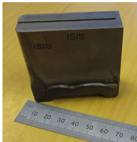
Figure 3.5. – Unirradiated ISIS TS-1 slab that has been cut in two, showing a hole drilled for a thermocouple. The tantalum cladding on the tungsten (1-2 mm thick) is visible.
