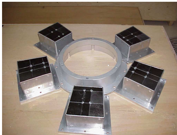
Figure 5.8. – Photo of the TOSCA HOPG crystal monochromators. Courtesy of ISIS Engineering Group.
