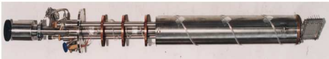
Figure 8.1. – The aluminium centrestick for use on TOSCA. On the right hand side, one can see the attached squared sample cell.
