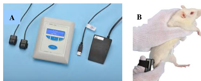
Figure 11: PAM device ( panel A ); force transducer on the operator's thumb ( panel B ).
