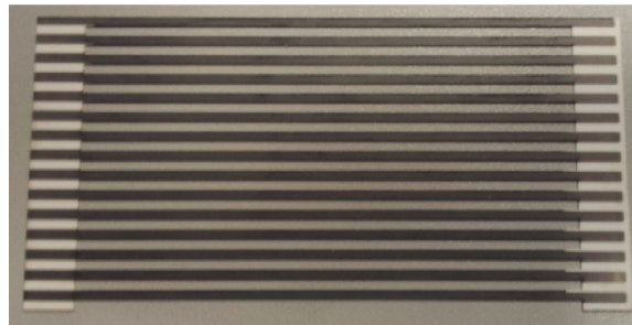
FIGURE 4.2: Photo of an \text{Al}_2\text{O}_3 lamella ( 10 \times 6 \text{ cm}^2 ), coated on both sides with a 1 \mu\text{m} thick ^{10}\text{B}_4\text{C} layer. The lamella is composed by 15 2 mm-wide strips. The space between the strips is 2 mm.
