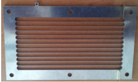
FIGURE 5.2: Aluminium grid used for the 3D converter of the new BAND-GEM prototype. The frame hosts some holes for grids alignment.
