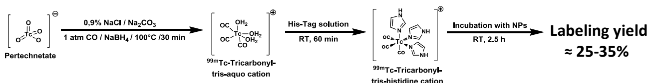
Scheme 2.2 Schematic representation of the three-steps radiolabeling protocol for SiNP-NTA and SiNP-NTA-TZ preparation.
