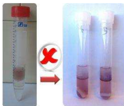
Figure 4.2. PEGylated DDT-GNRs (PEG-SH, MW. 5000 g mol -1 ) and DDT transfer to chloroform. Some gold nanoparticles (black/purple) were lost during the phase transfer for the insufficient amount of ligands.
