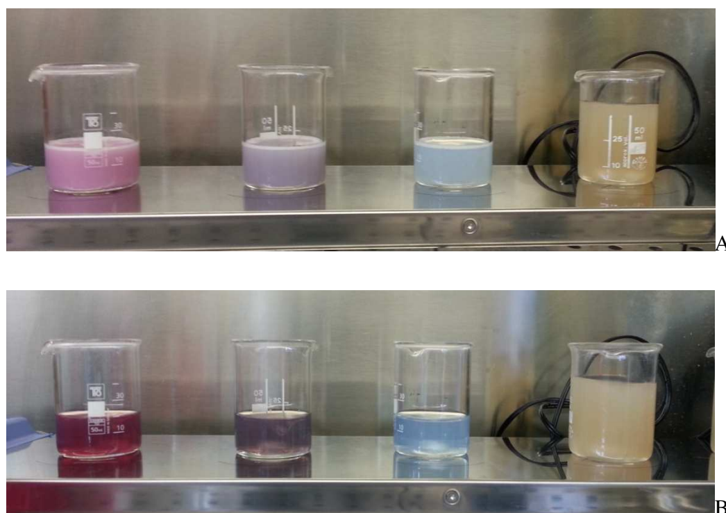
Figure 4.4. Photos of PLGA@GNPs, @GNRs, @GNCs and @MnO NPs after (A) 30 minutes and (B) 3 h after reaction has been started, respectively.
