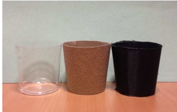
Figure 21 – The coatings used to cover the plastic cups. Starting from the left plastic, sandpaper and satin
