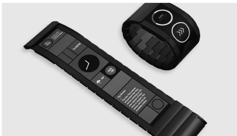
Figure 1.2: Polyera Corp.’s Wove Band, first example of completely printable and flexible electronic device based on organic semiconductor technology. The inventor A. Facchetti won the American Chemical Society’s National Award for Creative Invention 5 .
