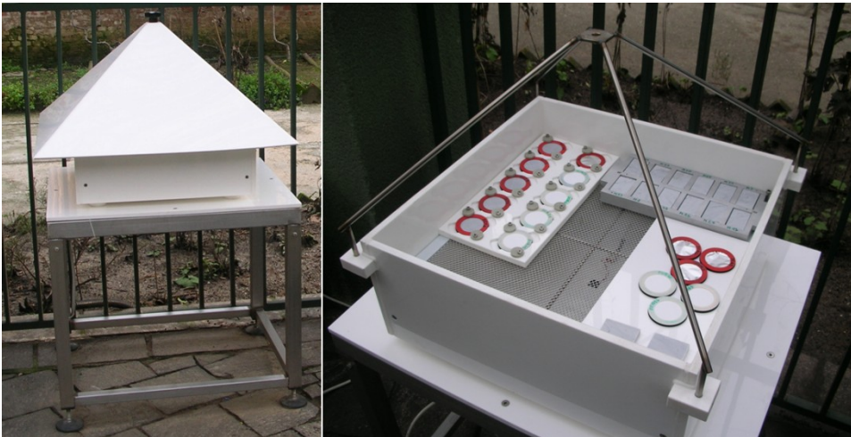
Figure 3.2: On the left, the external feature of the “deposition box”. On the right, the inside of the box, with some samples arranged on the exposure floor.
