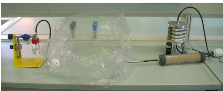
Figure 4.13: the Aerosol Generation Unit.
