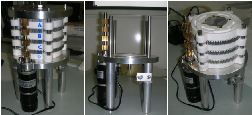
Figure 4.4: Prototype of the rotating cascade impactor. On the left, the assembled prototype is shown. The external structure is shown in the centre. On the right, the head cap removed allows to better see the assembling of the stages.
