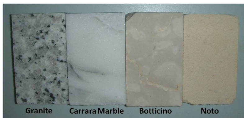
Figure 3.6: stone specimens before the exposure in depbox
