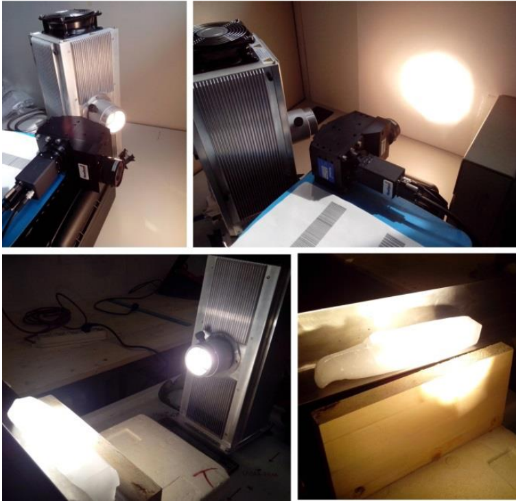
Figure 4.4: Set-up of the lamp tests. The images below show the sample of ice core lighted by the lamp.
