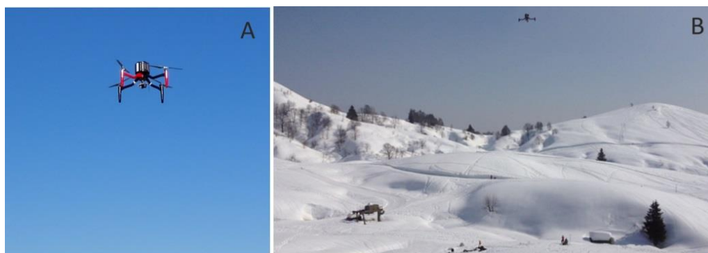
Figure 1.5: UAV in environmental research. A) Anteos UAV produced by Aermatica S.P.A. B) Use of the UAV in snow covered area during a field campaigns organized to measure spectral reflectance of snow after mineral dust depositional events (Di Mauro and others, 2015).
