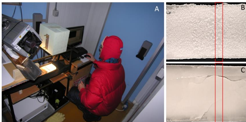
Figure 4.5: Collection of hyperspectral ice core data in cold room laboratory (A). Sampled firn core (B) and ice core (C) with the indication of the area where the measure were collected (red box).
