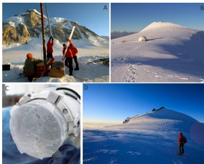
Figure 1.2: Ice core drilling to climate studies. A) A 2 meter section of ice core from Combatant Col (British Columbia) is removed from an electrothermal drill. Credit: Doug Clark, Univ. Washington. B) The drilling dome built near the summit of Mt. Ortles. Four 60-75 m deep ice cores were retrieved at an altitude of 3860 m. Credit: Paolo Gabrielli. C) Drill head and ice core from a depth of 2,874 meters at Dome C Station in East Antarctica. This ice core is about 491,000 years old. The entire core contains a continuous record of greenhouse gases for the past 650,000 years. Credit: Laurent Augustin. Laboratoire de Glaciologie et Géophysique de l'Environnement. D) Colle Gnifetti drilling sites, Monte Rosa Massif. Credit: Stefano Roverato.
