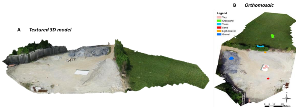
Figure 3.15: Textured 3D model created with SFM algorithms (A) and orthomosaic of the test site with the location of the spectra collected with the HyUAV (B, points dimension reflect the estimated footprint of the spectrometer).
