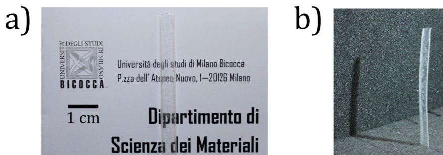
Figure 5.33: a) Photograph of the PVA film loaded with nanoemitters, macroscopically transparent. b) Photograph of the PVA film showing its self-standing properties.
