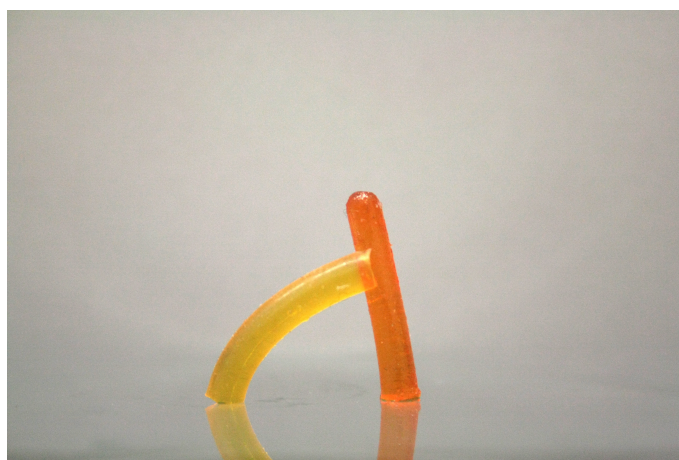
Figure 1.5: Photograph of PBA:EGDMA (4.5% v/V EGDMA content) self-standing bulk-samples. On the left the yellow sample loaded with the pivaloyl-derivative; on the right the orange sample loaded with the acetylated-derivative.
