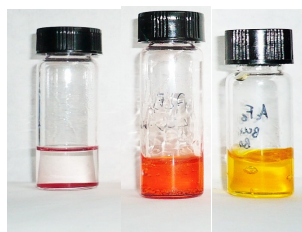
Figure 4.38: LEFT: Photograph of a 10^{-3}\text{M} solution of carminic acid in a BA solution. Phase separation is clearly visible. CENTER: Photograph of a 10^{-3}\text{M} solution of the carminic acid acetyl-derivative ( 5 ) in a BA solution. RIGHT: Photograph of a 10^{-3}\text{M} solution of the carminic acid pivaloyl-derivative ( 6 ) in a BA solution.
