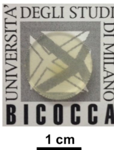
Figure 5.17: Photograph of the disk of transparent bulk PMMA obtained by bulk polymerization of 1.3 ml of MMA and 0.93 mg of radical initiator (AIBN), mixed with 43 mg of purified TiO 2 -loaded HD@pPMMA nanocapsules dry powder (sample name B69). In the centre of the sample a refractive index of 1.50 was measured at 633 nm. Please note that the refractive index for pure PMMA is 1.48.
