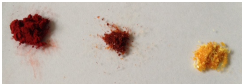
Figure 4.35: LEFT : Photograph of the dry powders of carminic acid (red, labelled 2 ). CENTRE : acetylated derivative (orange, labelled 5 ). RIGHT : pivaloyl-derivative (yellow, labelled 6 ).
