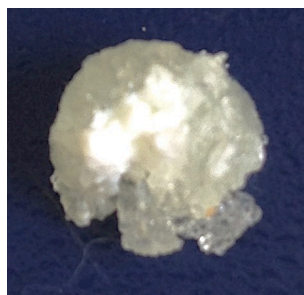
Figure 3.9: Representative photograph of the 156 nm NPs samples after the first DSC cycle from 273 K to 473K confirming that the exothermic peak in figure 3.7 is due to NPs syntherization. Signs of melting and powder syntherization are clearly visible particularly at the borders.
