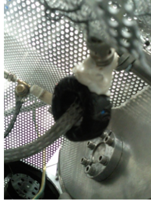
Figure 2.7: Rogowski coil located on the grounded side of the antenna directly measuring the current flowing inside the wire.
