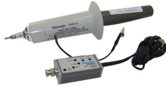
Figure 2.6: High voltage Tektronix P6015A probe, used to measure the voltage across the coil.
