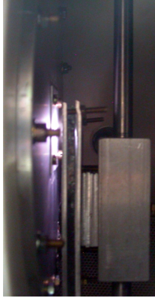
Figure 7.10: Photography of the \text{TiO}_2 thin film deposition over a wide area, moving the sample vertically.
