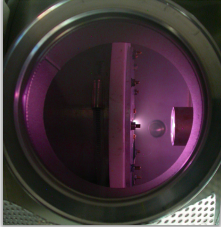
Figure 4.2: Photography of the supersonic jet exiting from the plasma source taken from the main quartz window facing the center of the deposition chamber. The QMS head is visible on the right, sampling the plasma jet.
