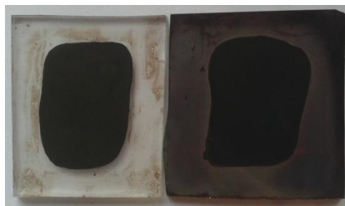
Figure 3. 19 Pictures of samples deposited on glass (left) and on Mo-coated glass (right) by dip-coating. The deposited area is 1.5x2 mm.
