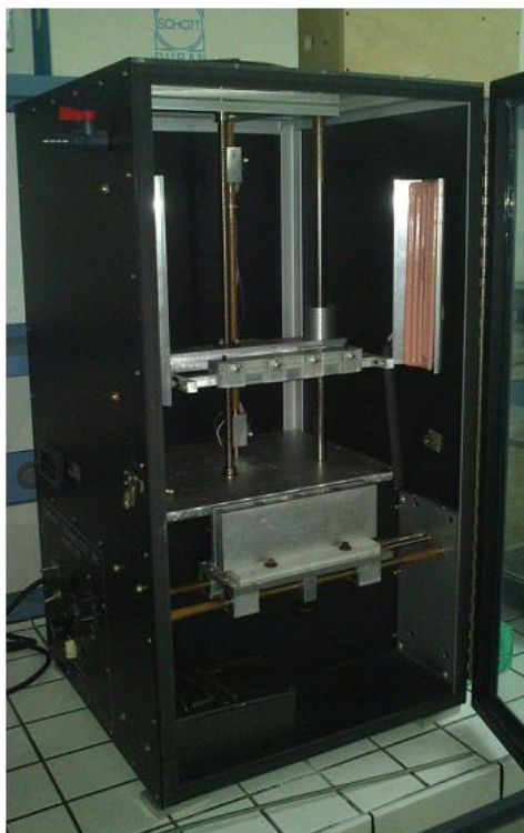
Figure 2. 3 Picture of the home built equipment used in this work for dip coating.
