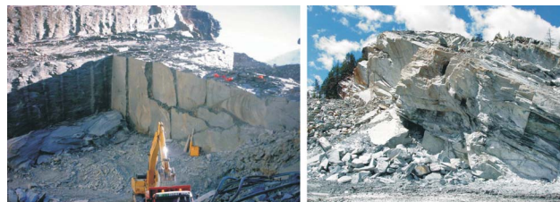
Fig. 2 Typical layout of a schistose (on the left) and massive serpentinite quarry (on the right, where also some tunnels of the abandoned chrysotile mines can be seen).
