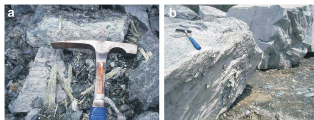
Fig. 4 (a) Quarry floor contaminated by chrysotile aggregates; (b) serpentinite block surface with chrysotile "beards".
